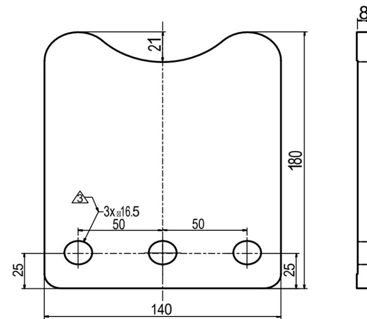
517044 Bracket plate, 3-hole, 150x195x8 mm, raw
