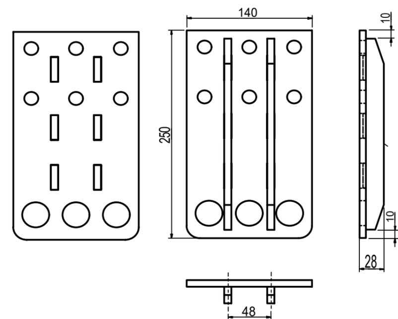
517095 Bracket plate, 140x150 mm, hot-dip galvanised
