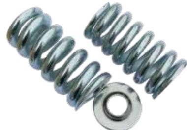
517142 Compression spring for chassis bracket, for vehicles from 15 tonnes,  $\varnothing 35/20$  mm, H70 mm, galvanised
