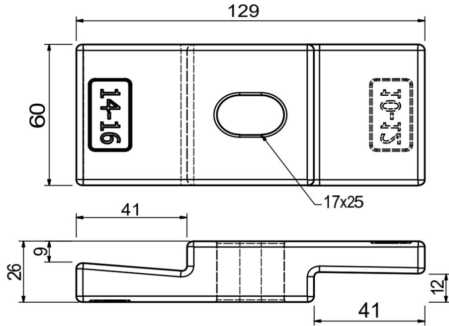
517025 Tensioning bracket, for 12 mm plate, galvanised
