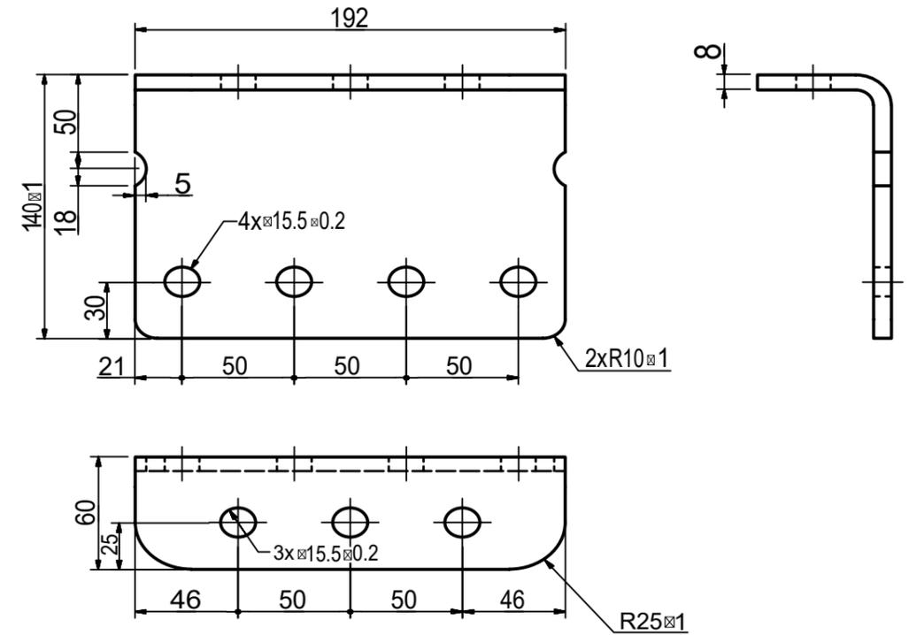
517122 Lower bracket, height 122 mm, 3-hole, galvanised
