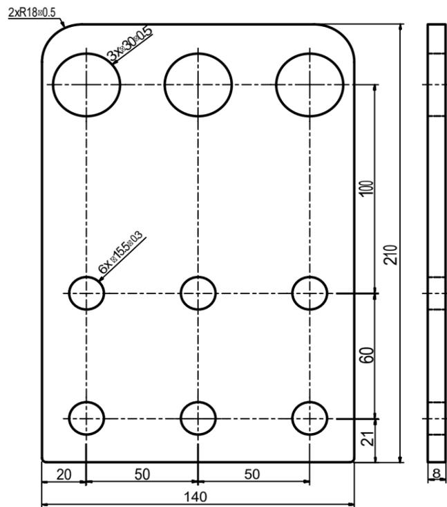
517124 Lower bracket, height 140 mm, 3-hole, galvanised
