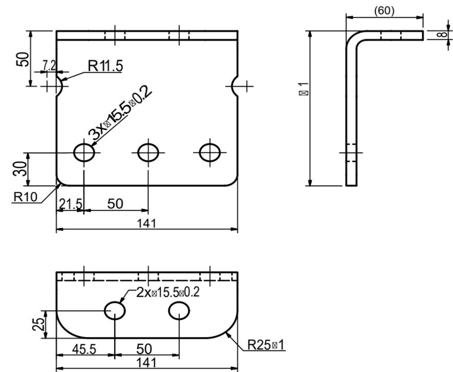
517136 Lower bracket, height 140 mm, 1-hole, galvanised
