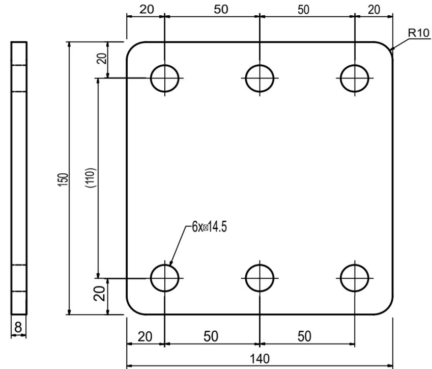
517196 Bracket plate, 6-hole, 140x150x8 mm, hot-dip galvanised
