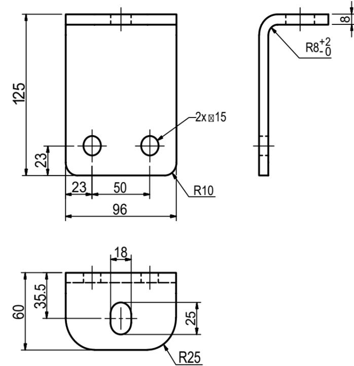
517138 Lower bracket, height 120 mm, 2-hole, galvanised
