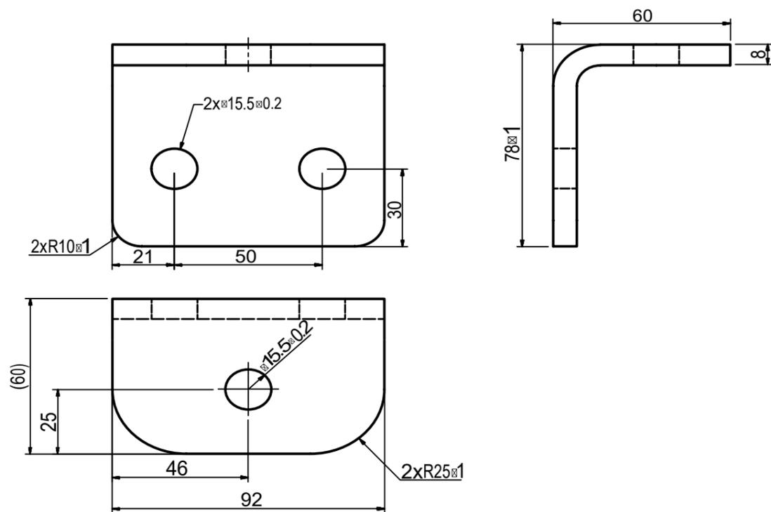
517134 Lower bracket, height 140 mm, 2-hole, galvanised
