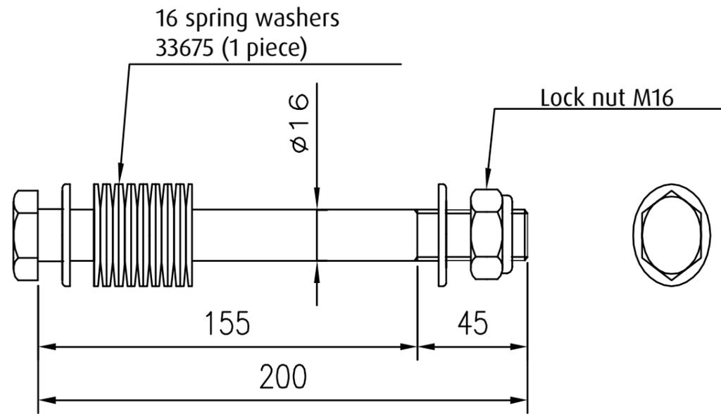
517019 Bolt set M16x160 mm, with 16 plate spring washers
