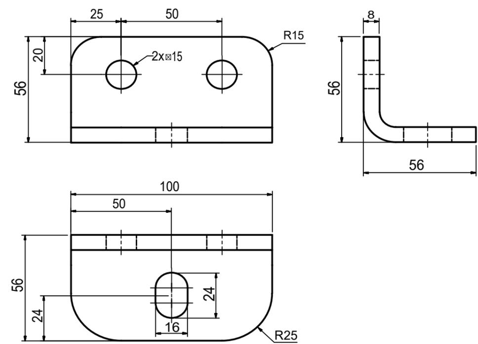
517101 Bracket, 56x56x8 mm, L: 100 mm, longitudinal hole, galvanised
