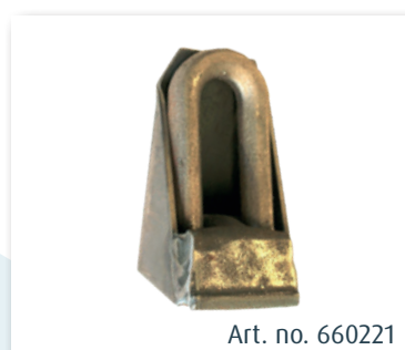
Lashing ring 8000 kg. 66x65x114 mm. Weight: 1,15 kg.
